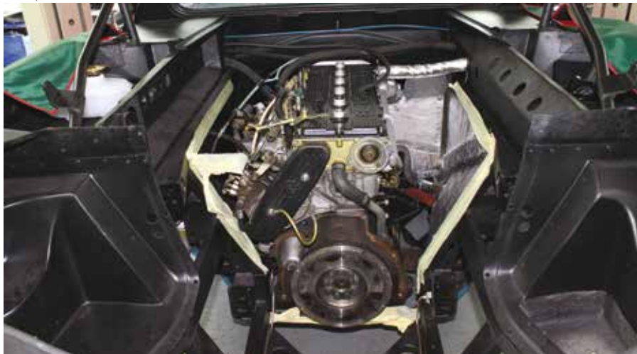
The inside of the engine bay is masked up to protect the newly restored interior from any minor scratches or damage as the engine is inched slowly into place.
