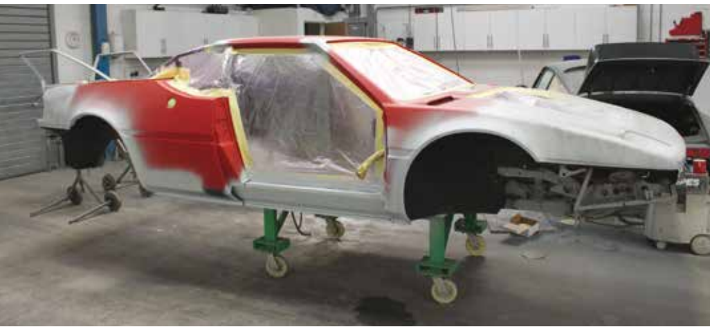
Finally the main car is primed and ready for painting. A base coat is applied for the colour followed by a clear PPG lacquer to give depth to the finish and protect the paint. A decision was made to use a modern paint process for longer durability and better finish
