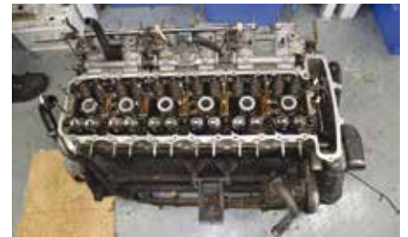
Meanwhile that fabulous M88 engine is tested, stripped and examined. Compression tests reveal poor figures so the decision is made to strip the head and investigate the reason. Closer examination reveals that the valves weren't seating properly due to excessive carbon build up. The valves were removed, checked and measured, cleaned and relapped.
