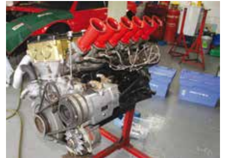
The engine can now be rebuilt using all new seals, gaskets and other ancillaries, with every component restored to its original factory finish. This is what a race engine looks like in a road car, complete with trumpets!
