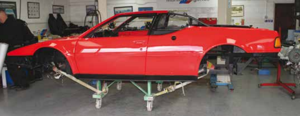
The painted shell arrives back in the main workshop on its specially adapted trolley. The refit can begin, but more than any other car the M1 is fragile in this state, so watch out! Is it a race car or a pick-up truck?
