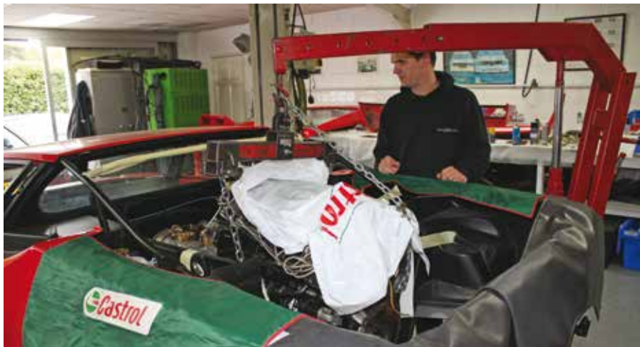
The engine is hung on the hoist and gently lowered in to the engine bay. This takes an inordinate amount of time to guide correctly, and three men. As the engine strains on the chains of the hoist, it is raised past the fragile fibre glass – freshly repaired and painted – rear panels.
