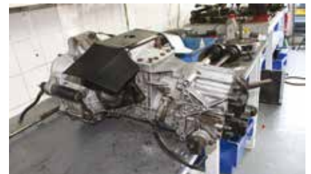
The transaxle - gearbox and differential - are now ready to be mated, having been fully overhauled, resealed and refinished. Best not get that toothbrush mixed up at home!
