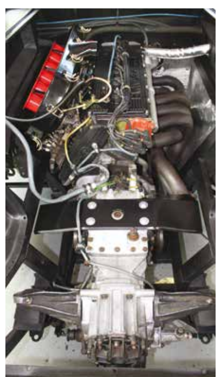
Finally the engine is seated precisely and can be mated to the transaxle. After a stressful stage in the project, the engine bay is starting to look complete as wiring and plumbing is carried out.
